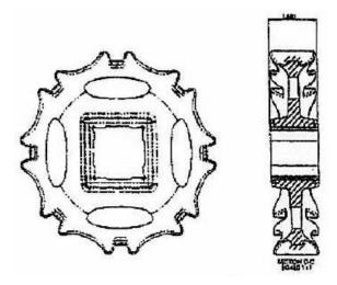
Figure #2 1.5"/2.5" x 10.5" sprocket, 13 tooth = 13/4 = 3.25. **Must have a timing mark.**
